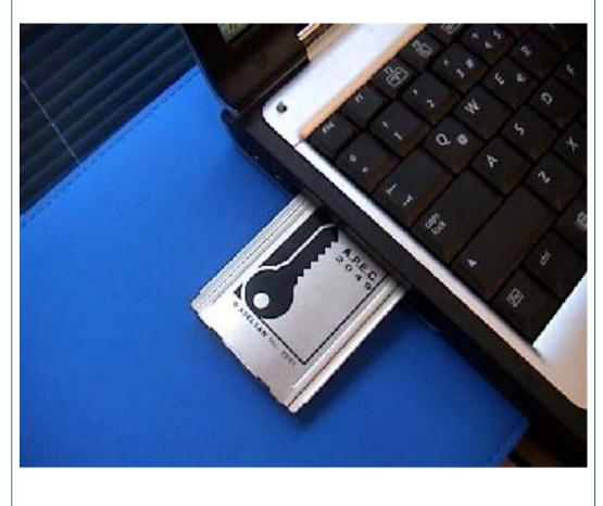
APEC is a cryptographic device developed to protect data classified as SECRET and below for storage and transmission. The device is primarily used for offline encryption of files on PCs. The stored and/or transmitted data security is managed by hardware encrypted PCMCIA card.
