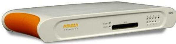
The Aruba 620 Branch Office Controller is a compact, cost-effective all-in-one networking solution. The 620 includes a firewall, wireless LAN controller, and nine-port Ethernet switch supporting four PoE+ ports. Aruba's centralized, zero-touch configuration and management model enables the 620 branch office controller to be deployed, monitored and controlled without any local IT staff. Additional deployment options include remote management or local configuration via a web interface.
