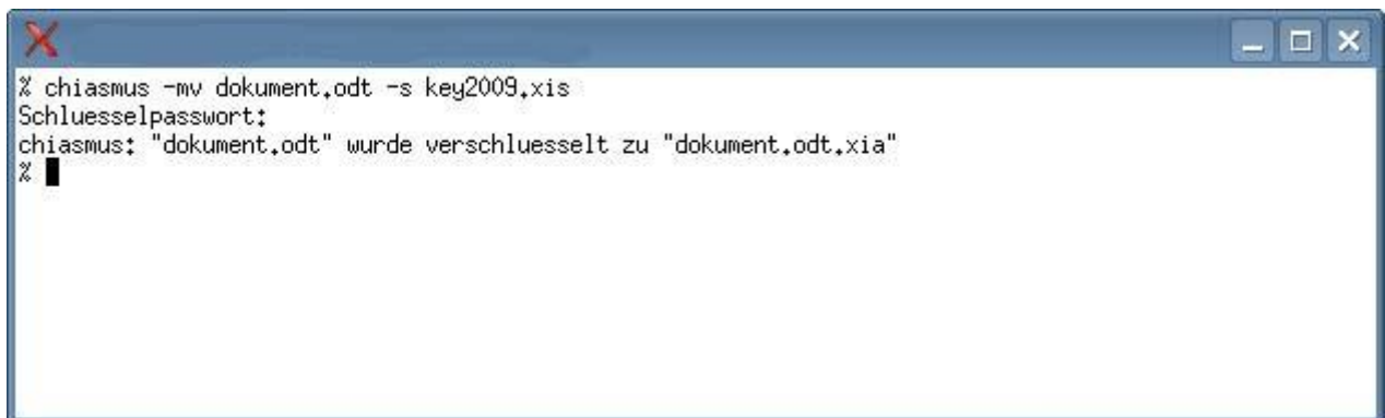
Figure: Chiasmus for Linux in operation. The Chiasmus user has enciphered the file dokument.odt with the keyfile key2009.xis. The password is not displayed on the screen.
