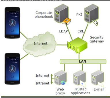
**Hoox m2** terminals are remotely connected to different servers in the organization to access messaging, Web proxy or other corporate servers.
