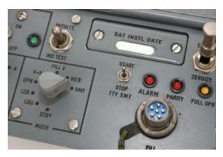
In order to retain the stored keys when the KG-84 is powered down, a standard military 6V lithium battery is used, such as the BA-5372/U or equivalent. The battery compartment is accessible from the front panel and is visible in the image above.
