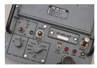
Compared to the KG-84A, the KG-84C had some interesting extras. It has a variable update counter, improved HF performance, out-of-sync detection (when in synchronous mode), asynchronous cipher text, plaintext bypass, and the European Telex protocol. When used with a suitable digital telephone unit, the KG-84 could also be used for secure voice transmissions.
