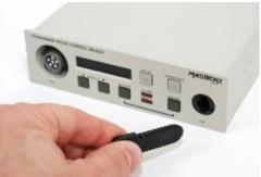
Due to miniaturisation of the KG-84, the KIV-7 was suitable for a wide variety of applications, ranging from modern PCs to submarines. Although the unit does not come in a ruggedised housing, it is very small and is fully complient with NSA TEMPEST requirements. This makes it ideal for space and load constraint environments. It only needs a single 5V power supply.
