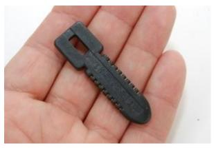
When crypto variables (i.e. the keys) are loaded into the KIV-7, the KIV-7 generates a random key that is used to encrypt the actual traffic encryption keys (TEKs). This random key is knows as the Key Encryption Key (KEK) and is stored inside the CIK. For this reason, the CIK is said to be *paired* with the device. The keys can only be retrieved by the KIV-7 if the appropriate CIK is present.
