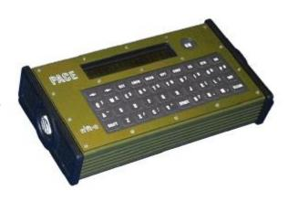
The device is housed in a water-resistant aluminium case, has a full QWERTY keyboard and a 16-character LCD screen. The built-in memory can hold up to 3800 characters of either plain text or encrypted text. The unit has built-in acoustic and optical modems, allowing messages to be transferred via virtually any medium, such as phone, radio, mail or messenger service. Full error correction is built-in allowing error rates of up to 10% and burst errors up to 37 consecutive bits.
