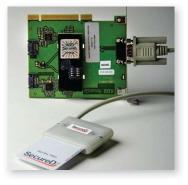
SecureD Desktop: A PCI card that integrates with existing SATA hard drives
